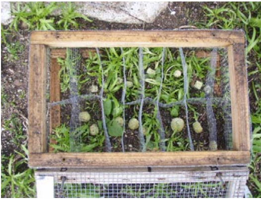
Fig. 1 Photo of bait degradation cage with pellets. Wire mesh bottom on this cage not visible in picture.
