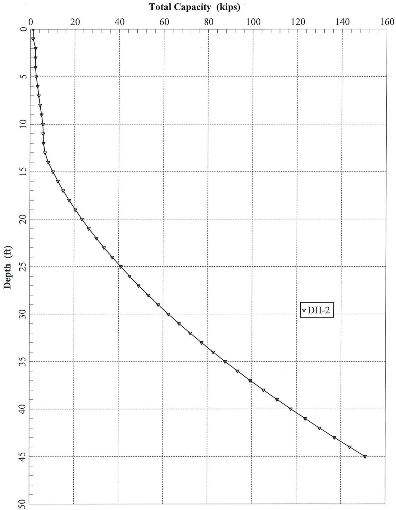
Total Capacity of pile vs. Depth
