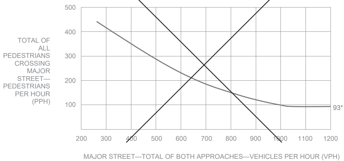
SPEED > 35 MPH Figure 4C-8. Warrant 4, Pedestrian Peak Hour (70% Factor)
