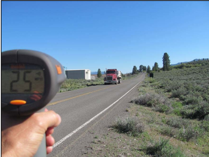
Figure 12 – Heavy Truck Passby Test Speed Monitoring.
