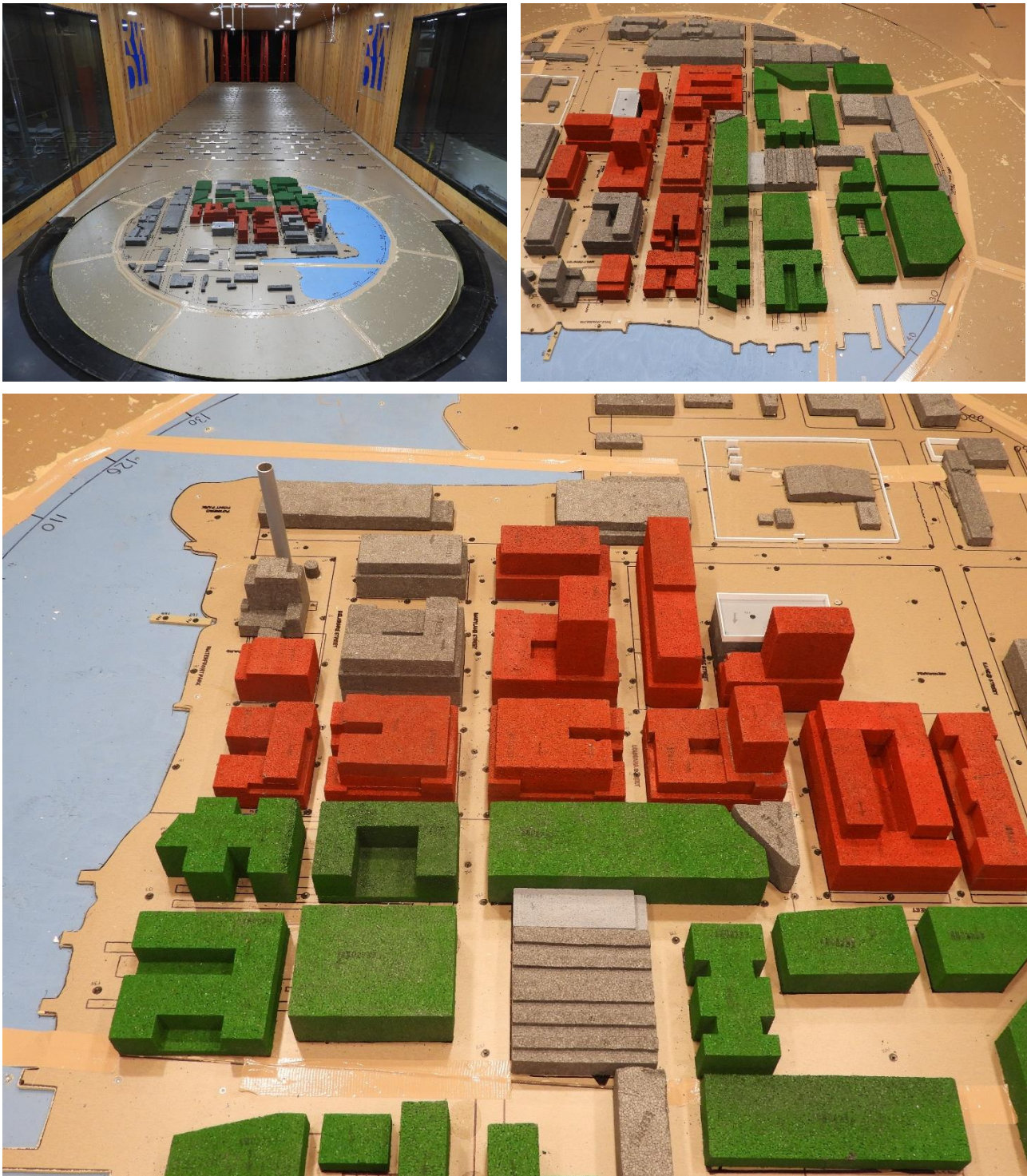
Image 2B: Wind Tunnel Study Model – New Project Variant B + Cumulative Configuration
