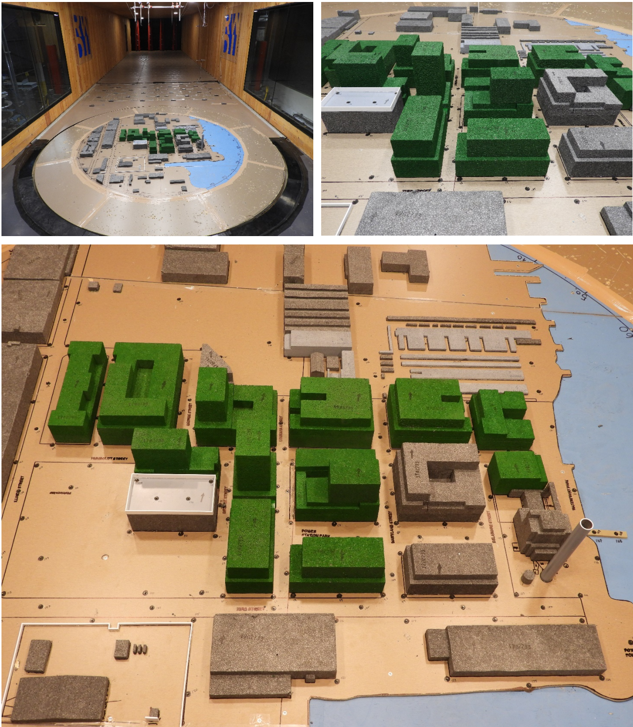
Image 2C: Wind Tunnel Study Model – Lower Heights Configuration
