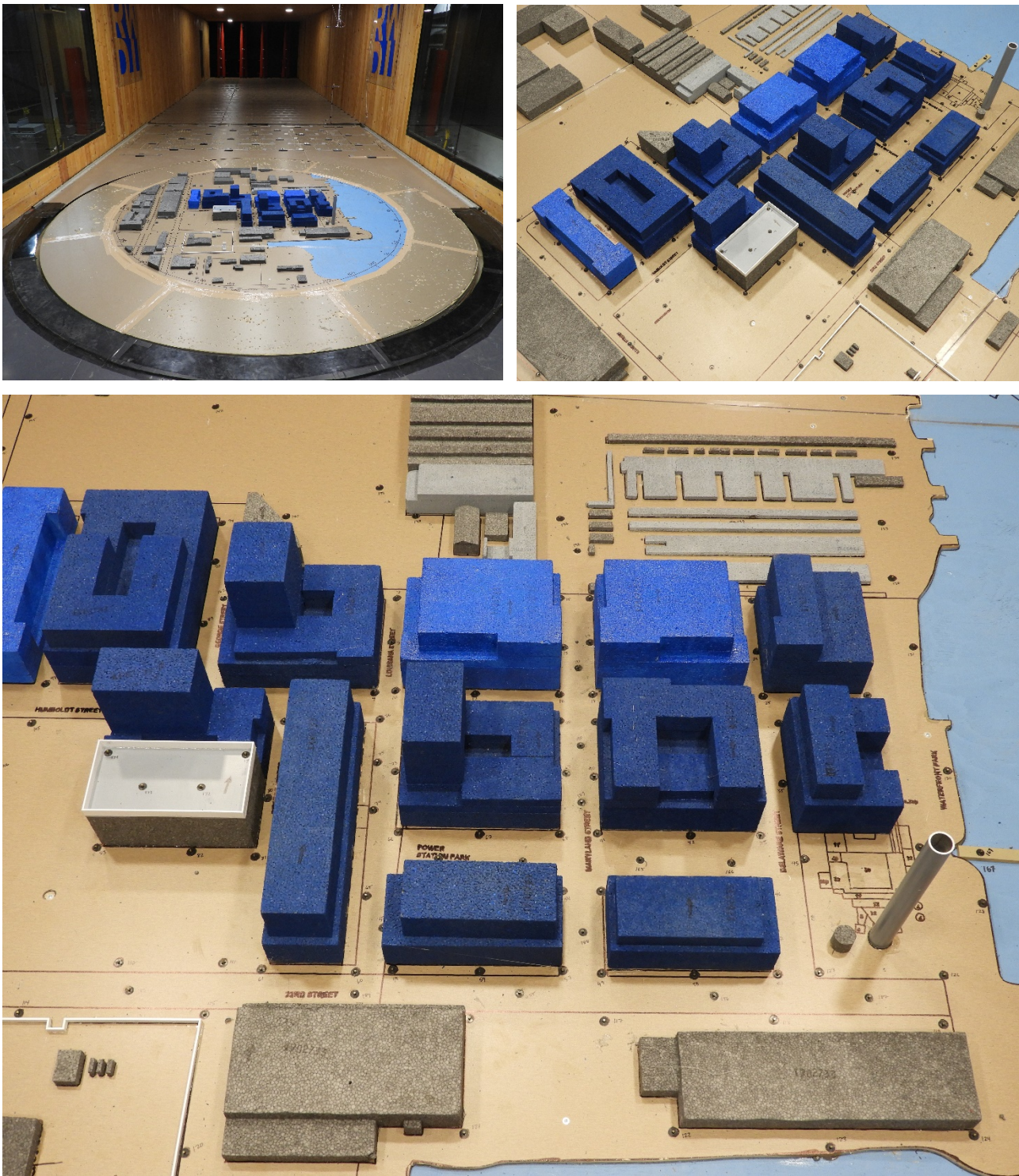
Image 2D: Wind Tunnel Study Model – Bulk Up Configuration
