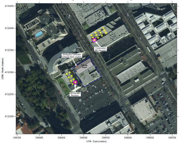
Figure 2.Project Site, Potential Locations for Emergency Generator, and Locations of<br/>Off-Site Sensitive Receptors and Maximum TAC Impacts
