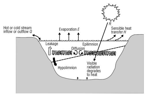
Source: Horne and Goldman 1994. Figure D-1. Horizontal Cross-Sectional View of the Physiochemical Processes and Stratification Layers Occurring in Lakes and Reservoirs
