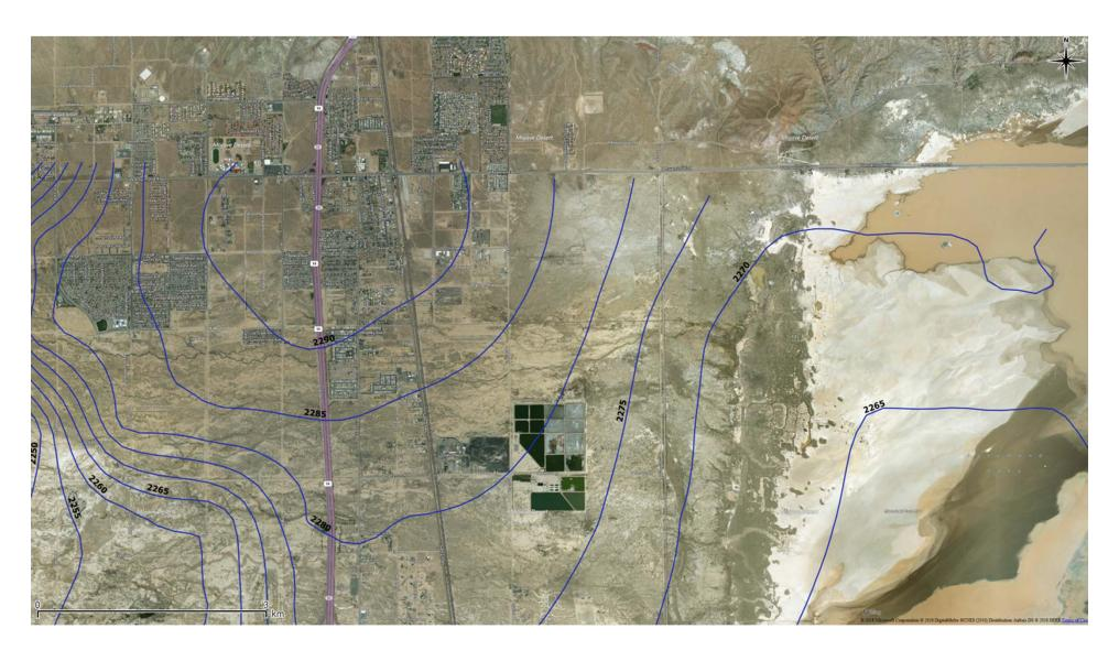
Figure 3: Simulated Water Table Elevation (ft above MSL) in USGS MODFLOW Model for the Antelope Valley at End of Calibration Period (2005)
