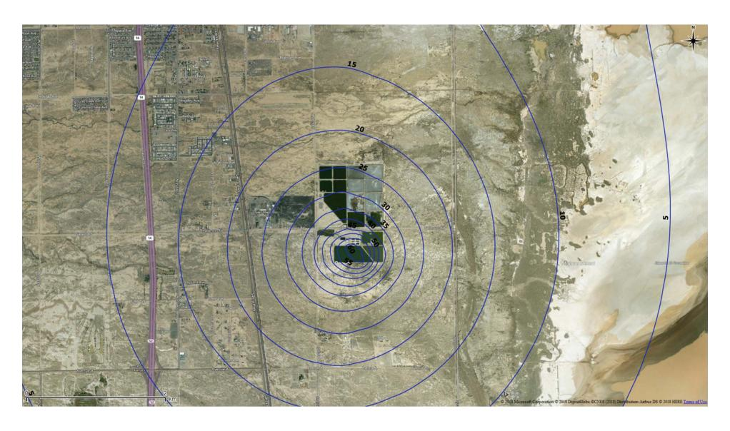
Figure 11: Groundwater Mounding Above Baseline (ft) Under Planned Design Changes for the RCSD WWTP
