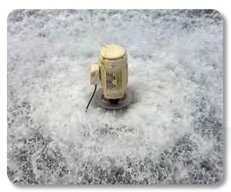
Aqua-Jet<sup>®</sup> aerator model SS-PW in operation in a TTHM stripping application.
