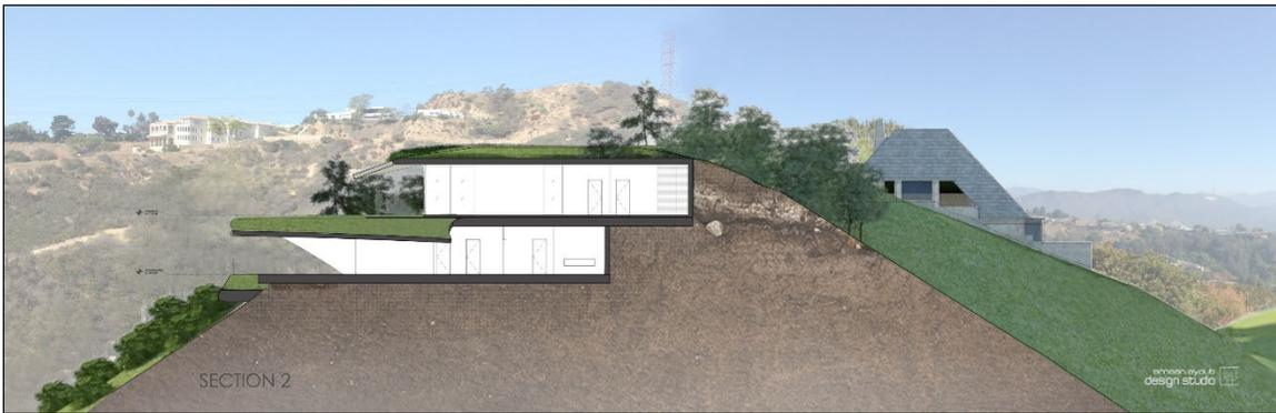
**Rendering 6:** Section view of the proposed new residence (left) and the existing Headley/Handley House at right, showing how the new residence will be sunken into the hillside.
