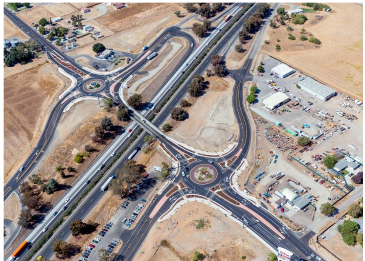
Roundabout interchange improvement at State Route 99 & Twin Cities Road.
