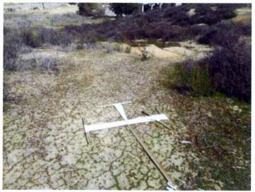
Photo #18: View of aerial survey marker located onsite
