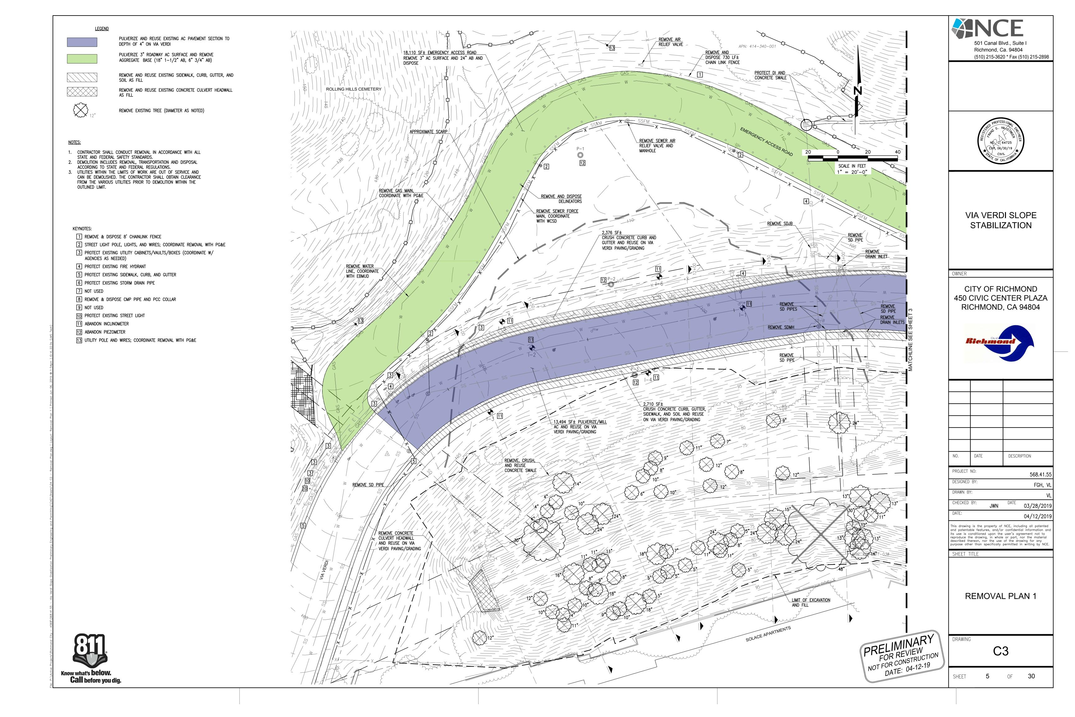
PULVERIZE AND REUSE EXISTING AC PAVEMENT SECTION TO DEPTH OF 4" ON VIA VERDI
