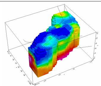
Figure 5- View is reverse of Figure 4 to better show the near-surface low-velocity layer draped on the fill terrace slopes, and the overall trend of increasing S-wave velocity with depth.
