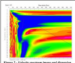
Figure 2 - Velocity spectrum image and dispersion curve (red dots) from Fill Terrace area
