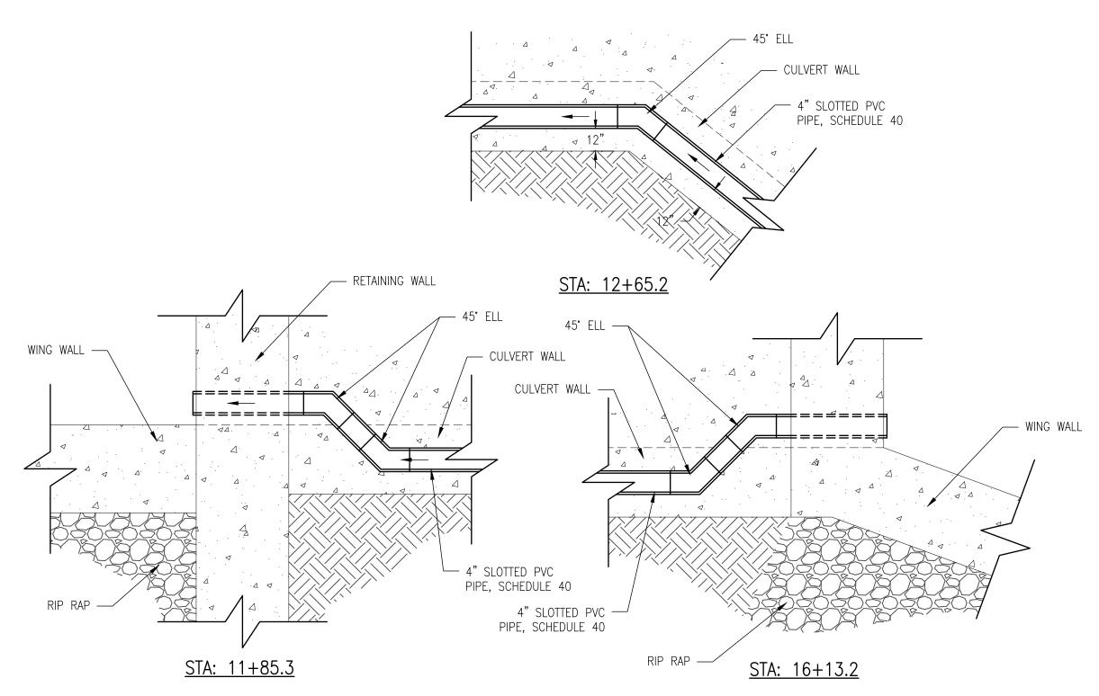
1 SLOTTED PVC PIPE DRAINS PLAN VIEW D1 N.T.S.
