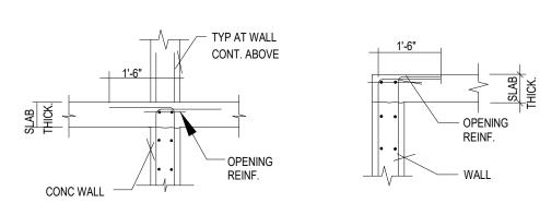
VERTICAL WALL REINF. DETAILS AT SLAB WHERE WALL IS DISCONTINUOUS
