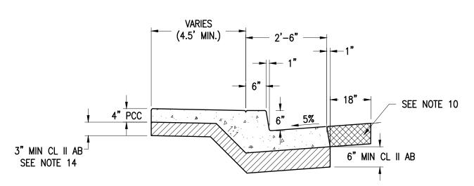
(3) TYPE A MONOLITHIC SIDEWALK WITH CURB AND GUTTER D4 N.T.S.
