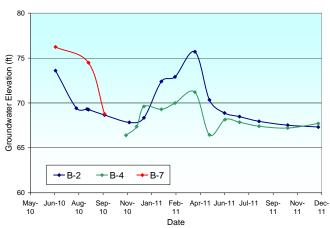
It is critical to observe that the peak groundwater level, which is very near the top of the culvert, is achieved in the April time frame, which is consistent with the collapse of the culvert on April 15, 2010.
