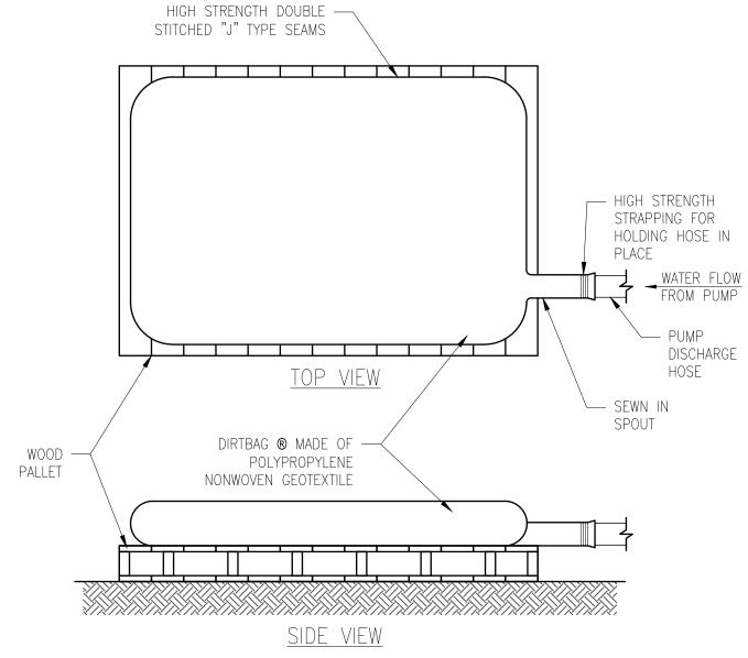
1. DIRTBAG SHALL BE MANUFACTURED PER SI GEOSOLUTIONS' SPECIFICATIONS OR APPROVED EQUIVALENT.
