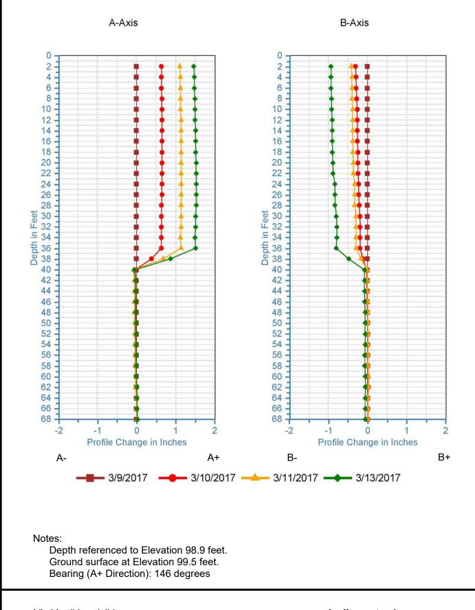
Via Verdi Landslide
