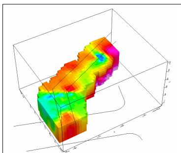
Figure 7 - Velocity block model viewed from same angle as in Figure 4 with more of the upper portion removed to show velocity configuration at the base-of-culvert (invert) elevation. Low-velocity layer is much less evident
