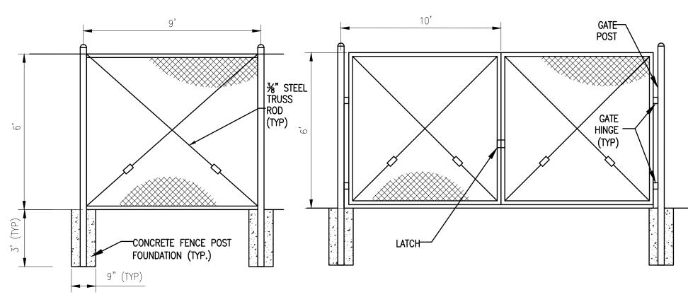
1. CHAIN LINK FABRIC SHALL BE ZINC COATED STEEL MANUFACTURED IN COMPLIANCE WITH ASTM STANDARD A 392 WITH A 2 INCH MESH OF 9 GAUGE WIRE WITH KNUCKLED SELVAGE.
