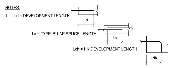
2. WHEN SPLICING BARS OF DIFFERENT SIZE, USE LAP SPLICE LENGTH OF LARGER BAR, UON
