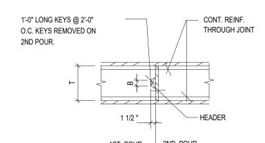
8 2 1/2 VERTICAL POUR JOINT IN SUSPENDED WALLS SHALL 10 3 1/2 BE WITHIN MIDDLE THIRD OF THE SPAN U.N.O. 12 5 1/2 >12 T / 2
