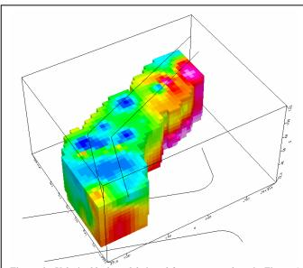
Figure 6 - Velocity block model viewed from same angle as in Figure 4 but with upper portion stripped away to show the S-wave velocity configuration at the top-of-culvert elevation. This view shows the deeper low-velocity layer is most pronounced at the bend in the culvert.
