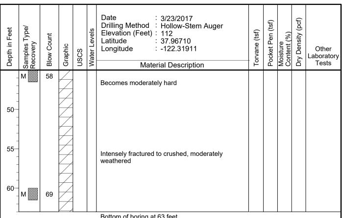
Bottom of boring at 63 feet No groundwater encountered Boring converted to Piezometer P-1
