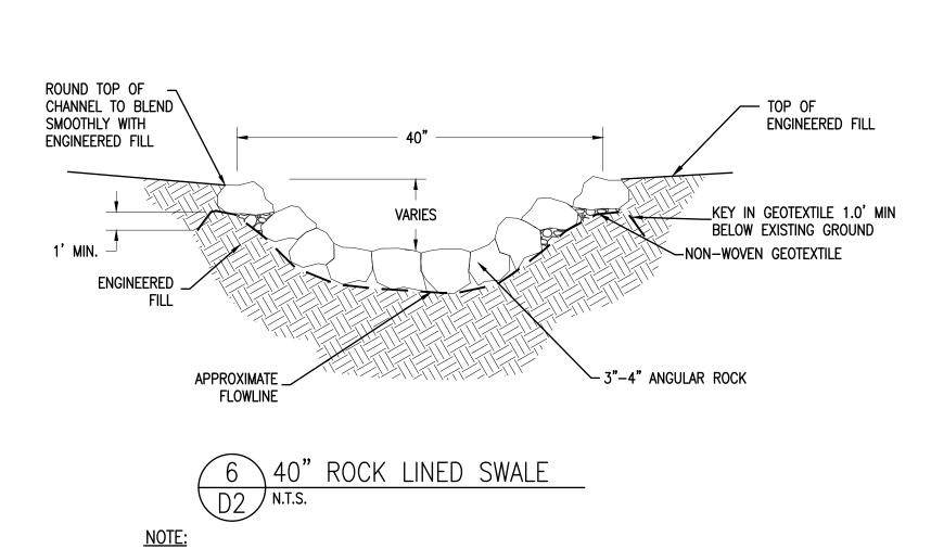
1. FLOWLINE DEPTH MAY VARY DEPENDING ON ENGINEERED FILL FINISH GRADING; SEE
