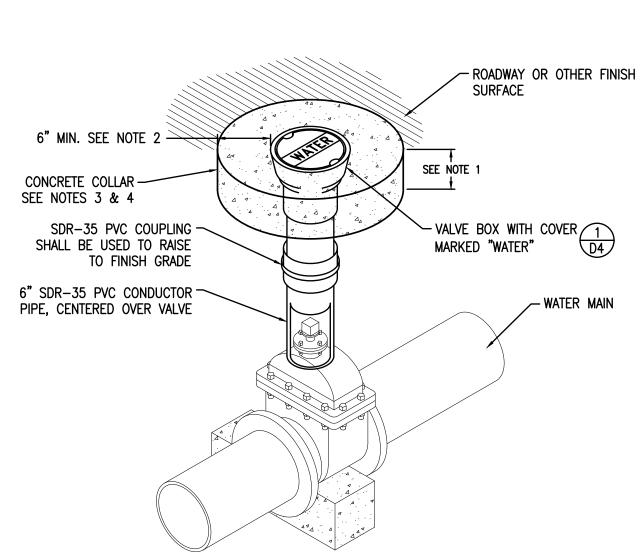
1. CONCRETE COLLAR SHALL BE MINIMUM 6-INCHES THICK OR MATCH PAVEMENT THICKNESS, WHICHEVER IS
