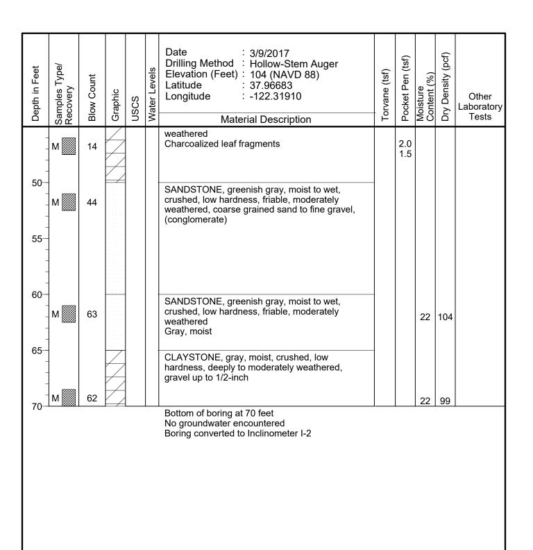
Via Verdi Landslide Richmond, California Log of Boring 2 (Inclinometer I-2) (Page 2 of 2)
