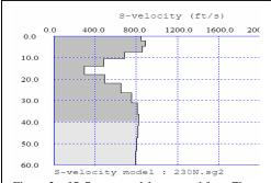
Figure 3 – 1D S-wave model generated from Figure 2 dispersion curve showing low-velocity "notch"
