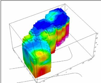
Figure 4 - Velocity "block" prepared from 1D S-wave velocity models, viewed from the south. Depth range shown is from the ground surface to the base of the culvert. Blue area indicates lower S-wave velocity associated with the shallow subsurface at the fill terrace. Culvert location is shown for reference.
