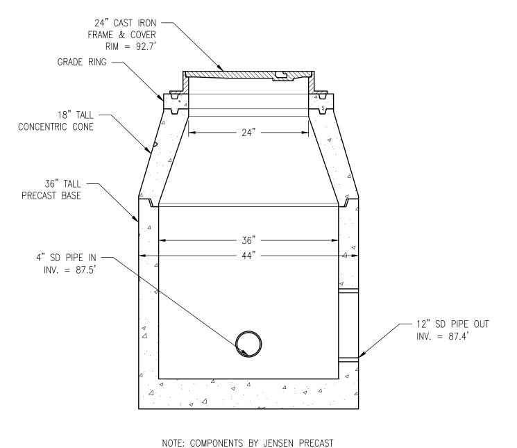
4 STORM DRAIN MANHOLE 1 DETAIL
