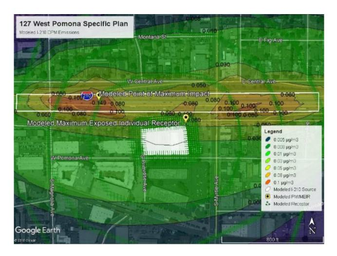
Figure 10: Modeled Source, Receptor, and DPM Contours
