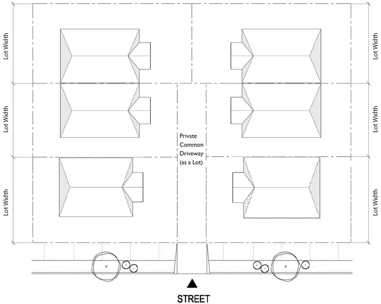
2. Where a compact lot is bounded by a T-shaped or an L-shaped private common driveway, the average lot width shall be measured as follows (see Figures 22.04.050-G and 22.04.050-H):
