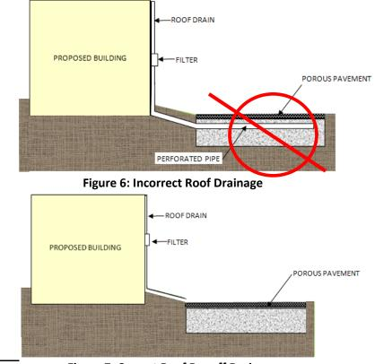
Figure 7: Correct Roof Runoff Drainage
