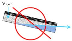
Figure 5: Incorrect Sloping of Permeable Pavement
