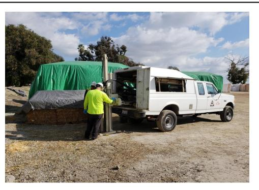
Photograph 3: Looking northwest at the site during direct push drilling of Boring B3.
