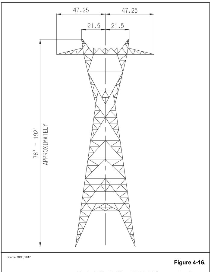
Typical Single-Circuit 500 kV Suspension Tower
