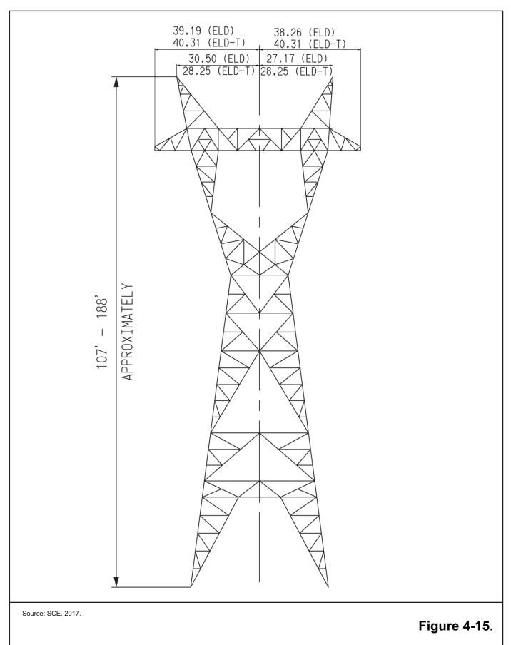
Typical Single-Circuit 500 kV Dead-End Tower
