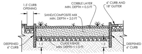
BIO-RETENTION CROSS SECTION & MODIFIED CURB SECTION
