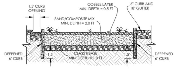
BIO-RETENTION CROSS SECTION & MODIFIED CURB SECTION
