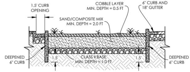
BIO-RETENTION CROSS SECTION & MODIFIED CURB SECTION
