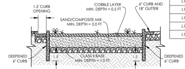
**BIO-RETENTION CROSS SECTION & MODIFIED CURB SECTION**
