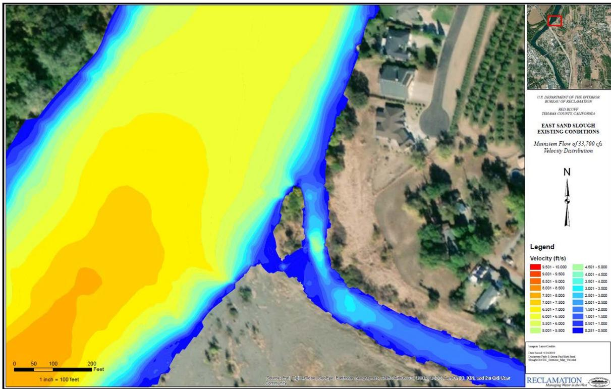
Figure 8. SRH2D Velocity results for existing conditions
