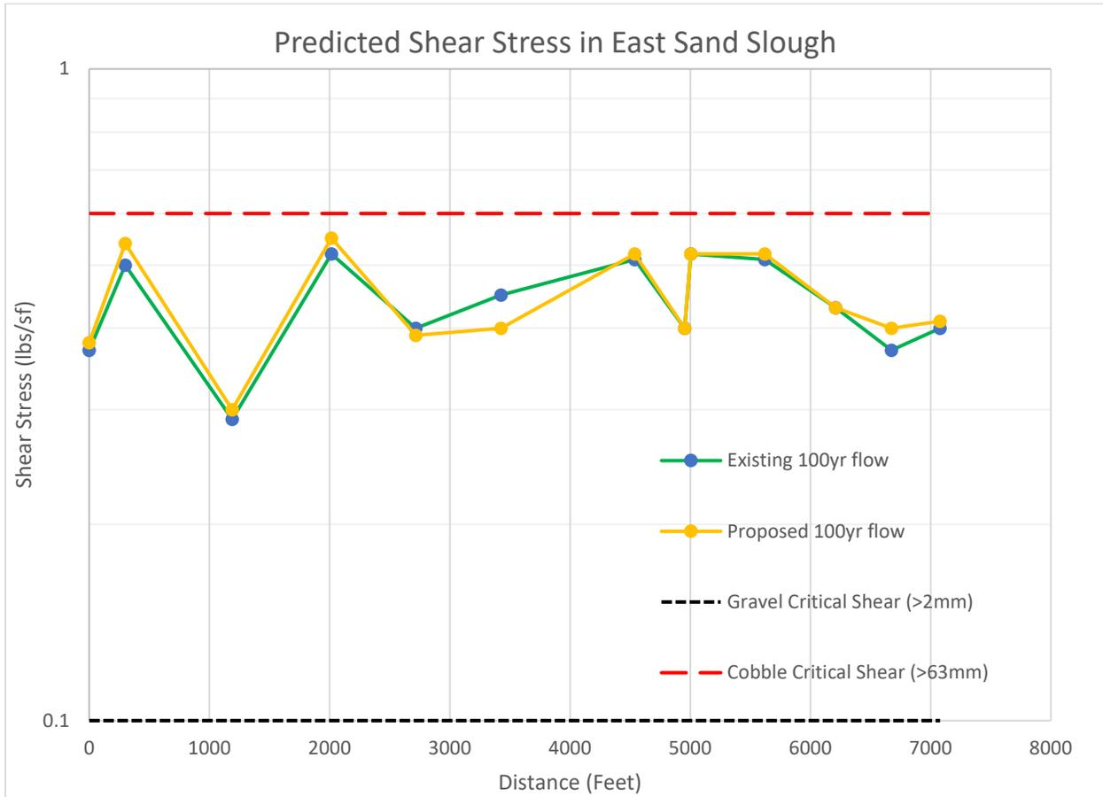
**Figure 4. Hec-RAS Shear Stress results**
