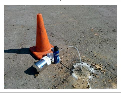
Subject: Soil gas sample collection using Difluorochloroethane (DFA)as a leak detection compound.
