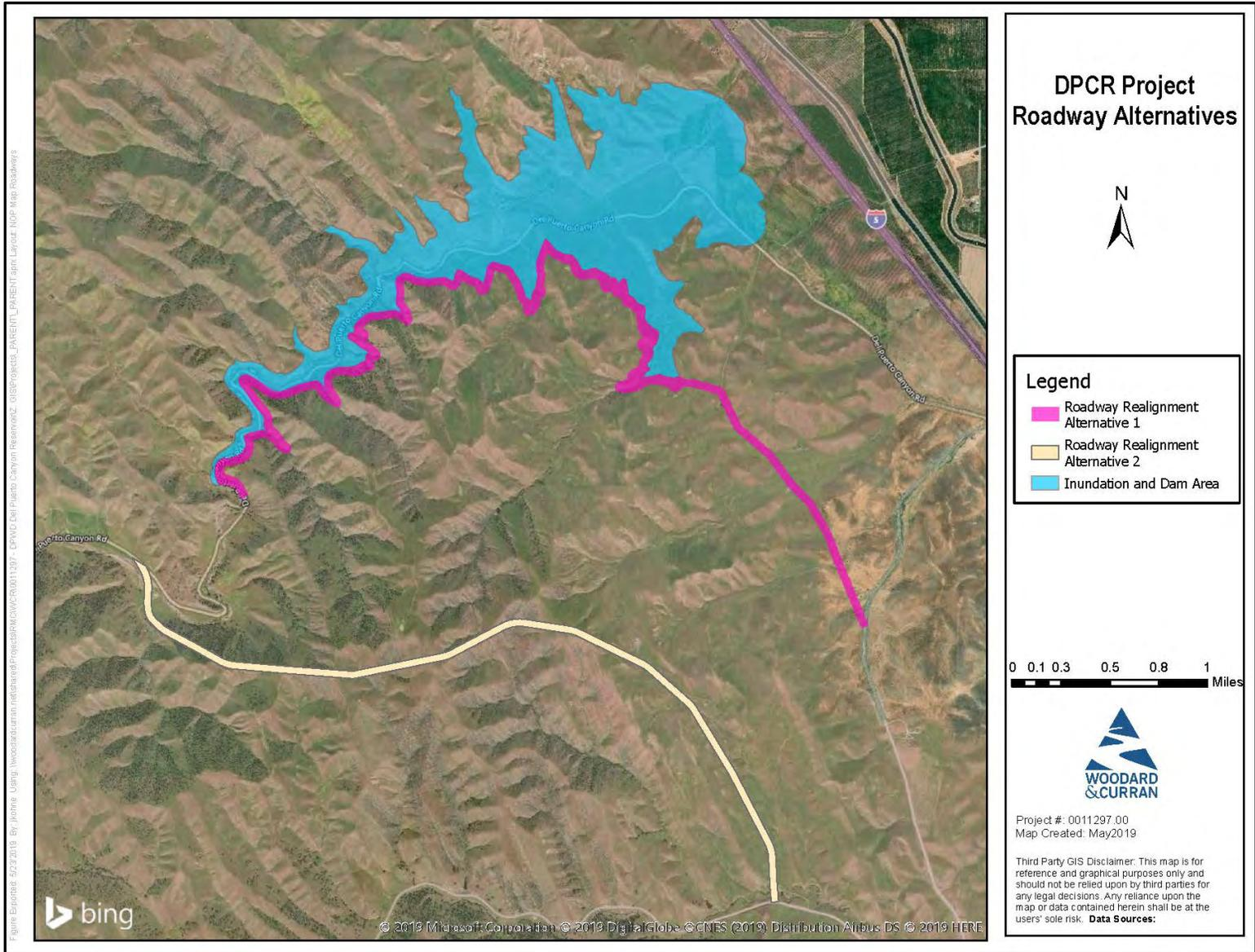
Figure 4: DPCR Project Roadway Alternatives. Project: DPCR Project, Parent: DPCR Project, Child: DPCR Project, Map: Map Roadways
