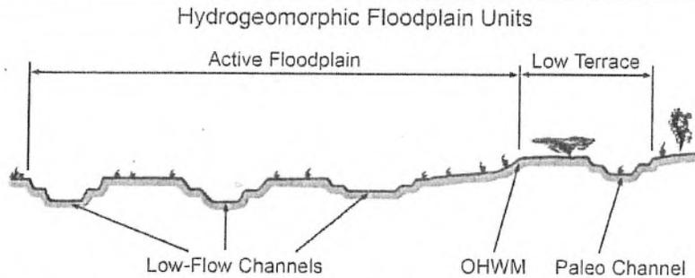
**Procedure for identifying and characterizing the floodplain units to assist in identifying the OHWM:**
