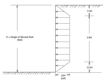
Diagram 1 – Earth Pressure Distribution for Tie-back or Braced Shoring Wall
