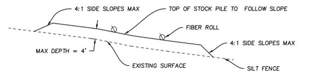
TYPICAL STOCKPILE SECTION A-A
