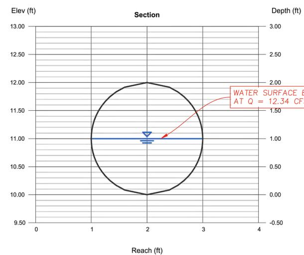
**G** 100 YR OVERFLOW PIPE CAPACITY CALCULATION
