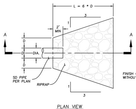
**C** RIPRAP APRON AT CULVERT OUTLET DETAIL
