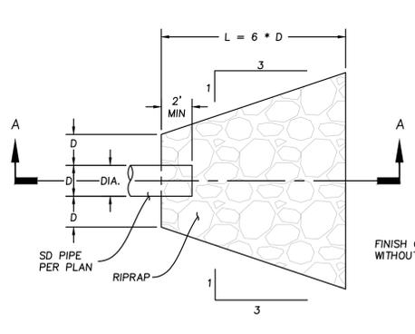
**C** RIPRAP APRON AT CULVERT OUTLET DETAIL
