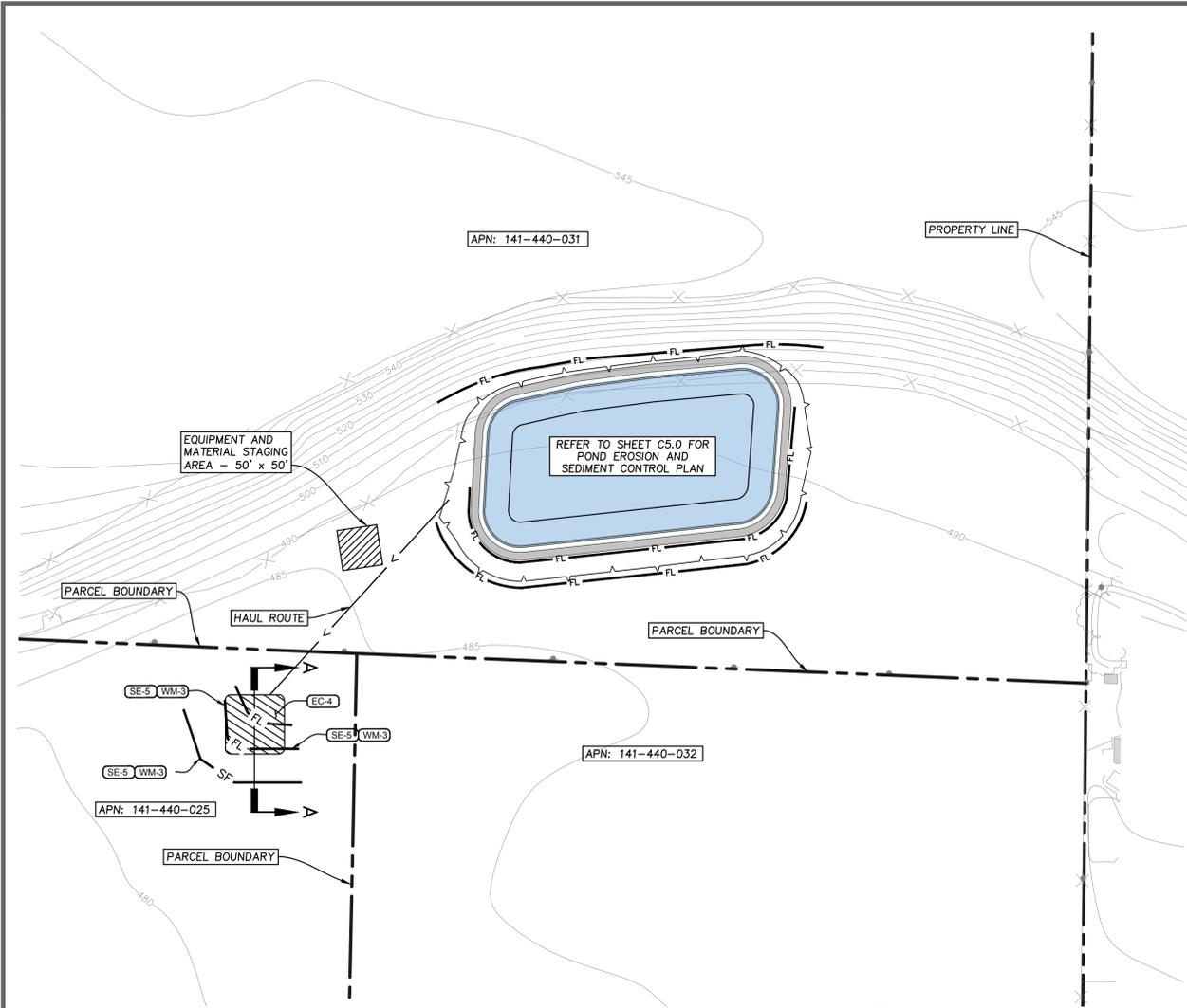
TEMPORARY STOCKPILE PLAN AND EROSION CONTROL
