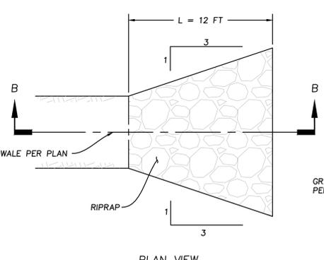
**E** RIPRAP APRON AT SWALE OUTLET DETAIL
