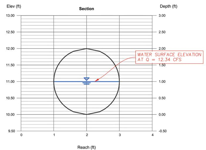
**G** 100 YR OVERFLOW PIPE CAPACITY CALCULATION
