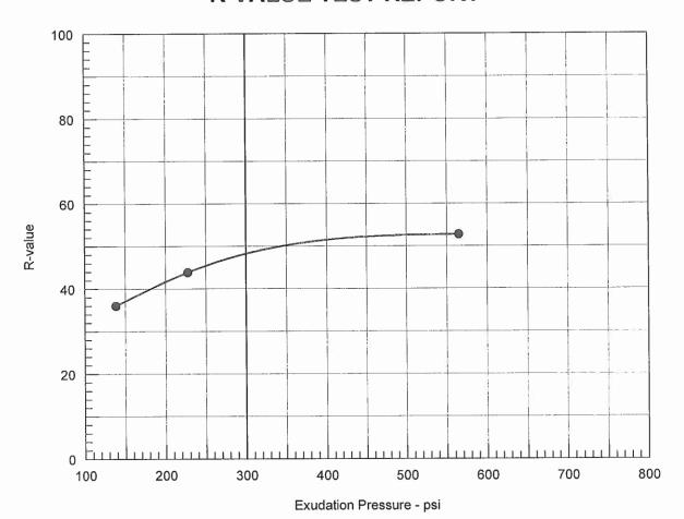
Resistance R-Value and Expansion Pressure - ASTM D 2844
