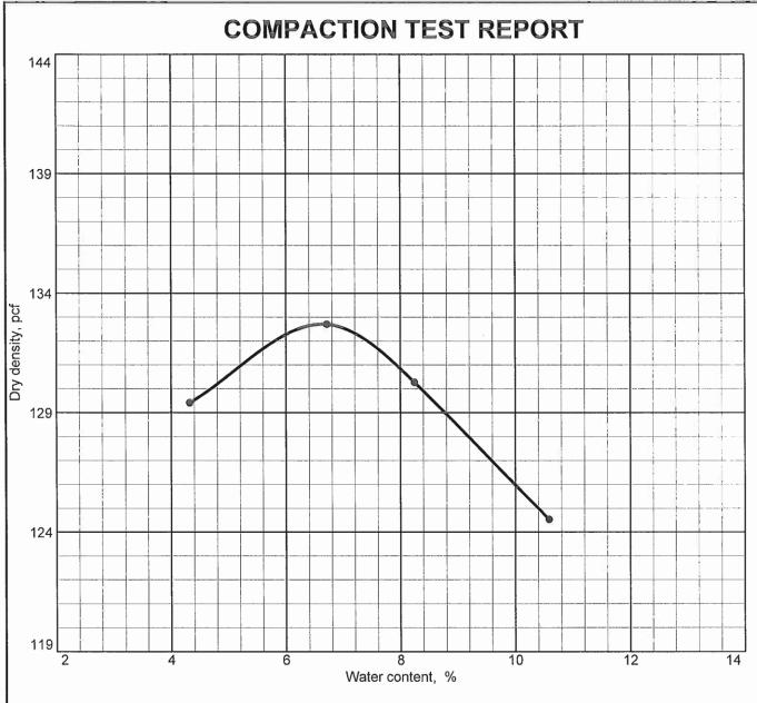
Test specification: ASTM D 1557-12 Method A Modified
