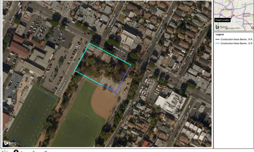
Figure 4-1. Location of Temporary Construction Noise Barriers
