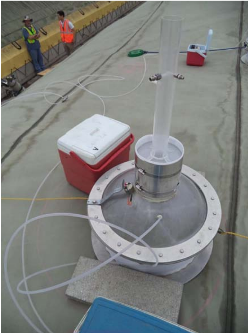
Photo 1. Flux Chamber Testing on the Gore® Cover.
