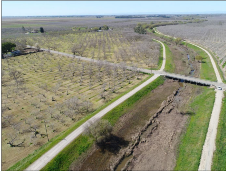
Aerial view looking downstream at Yankee Slough. Erosion damage occurs along the waterside toe of the right levee.
