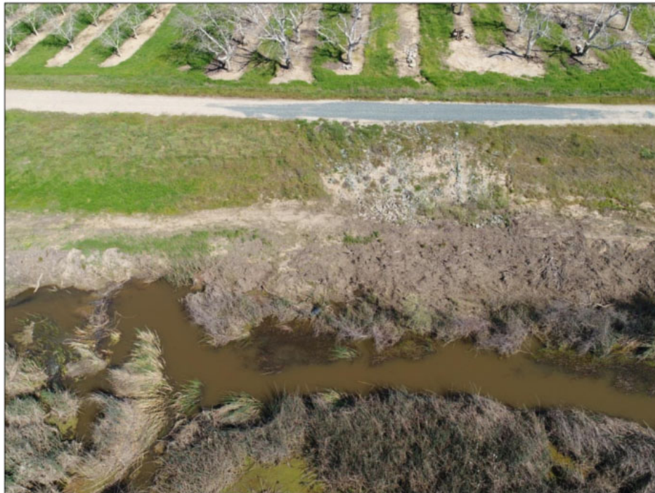
Aerial view looking at erosion site and emergency repair rock placement. Beaver dam crossing the main channel is visible in the left side of the photo.
