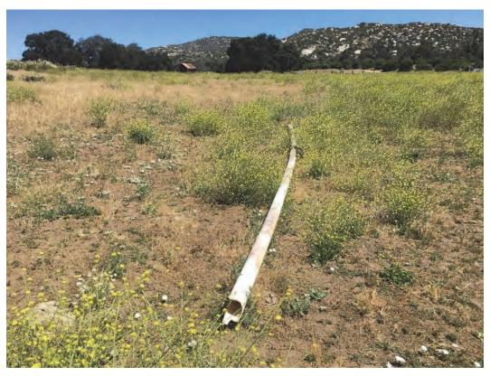
E-5. Broken polyvinyl chloride (PVC) pipe (06/13/2017).
