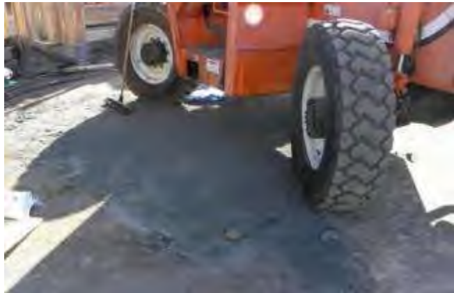
Hydraulic hose leak and absorbent deployment
