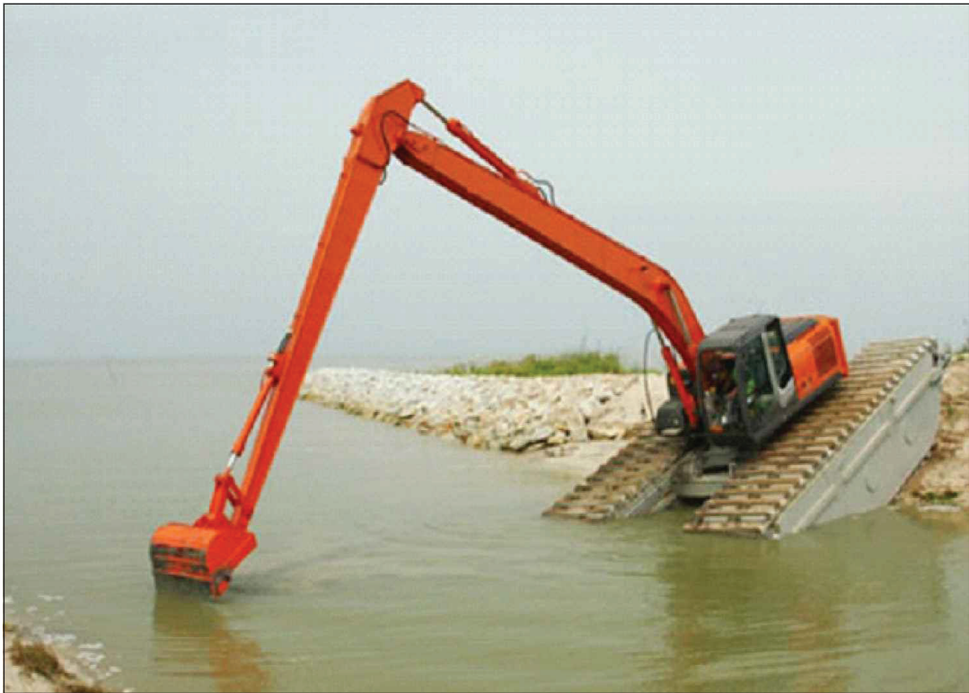
Amphibious long reach excavator: Long Reach High Reach Marsh Buggy
