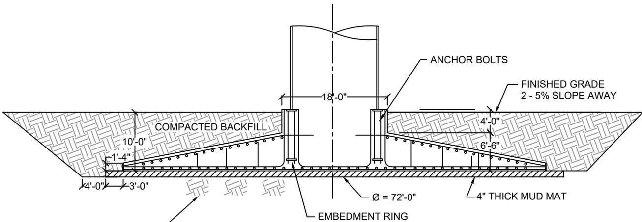
COMPACTED SUBGRADE. GROUND MODIFICATION (RAMMED AGGREGATE PIERS, OVEREXCAVATION OR RIGID INCLUSIONS) MAY BE NECESSARY TO ACHIEVE DESIGN BEARING
