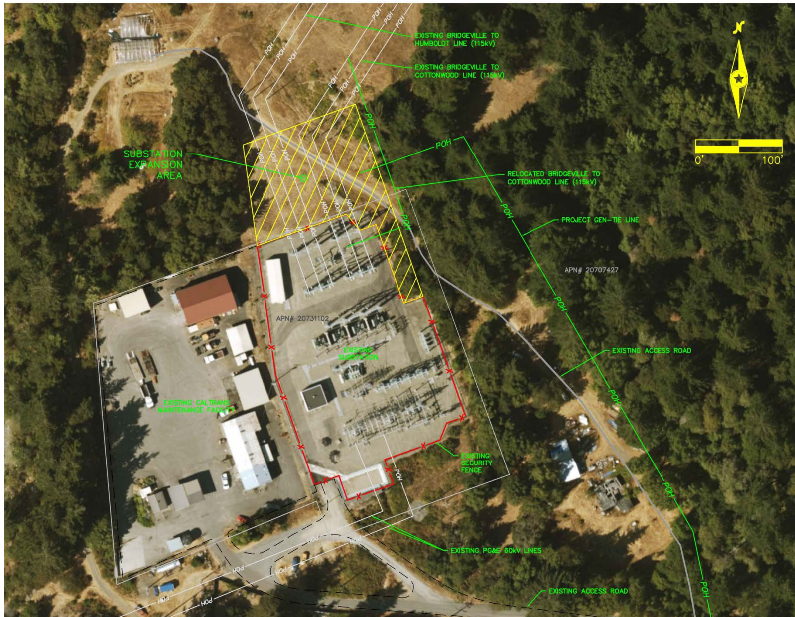
Figure 2-9. Gen-Tie Interconnection with the Pacific Gas and Electric Company Bridgeville Substation
