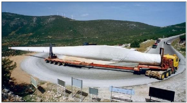
Figure 2-18. Clearance for Blade Tip Swing-out
