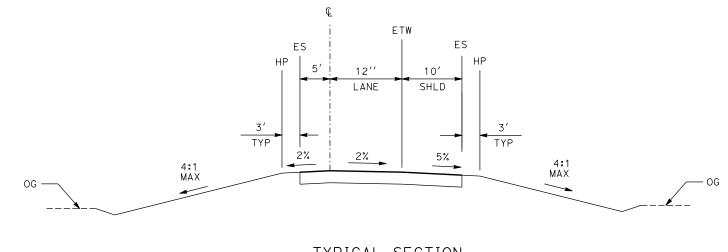
TYPICAL SECTION "WB ON RAMP" LINE @ SR 59 "WB OFF RAMP" LINE @ SR 59 "EB ON RAMP" LINE @ SR 59
