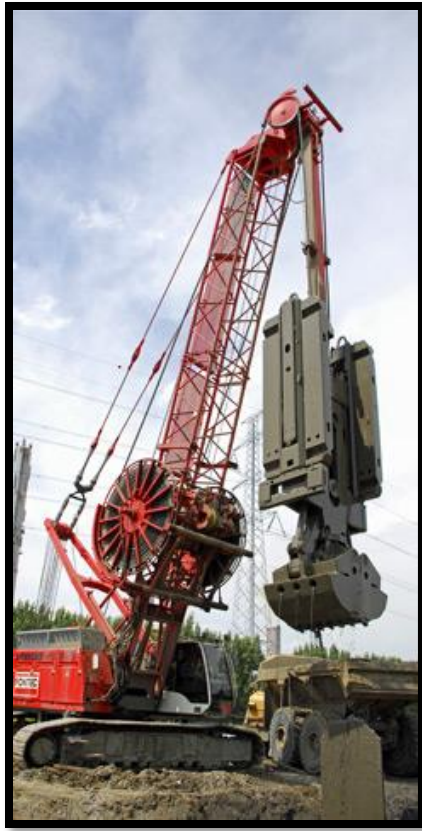
Figure 4. Cutoff Wall Excavation Equipment.
