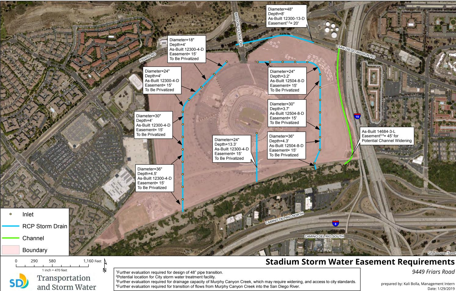
As-Built 14684-3-L Easement<sup>3,4</sup>= 45' for Potential Channel Widening
