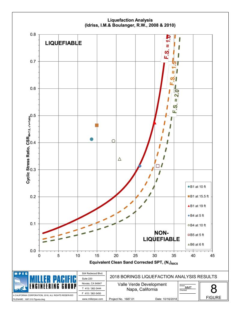
Liquefaction Analysis Utilizing Standard Penetration Test Data
