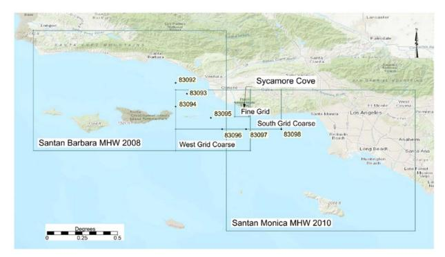
Figure 24: Regional digital elevation models used to develop the two coarse grids and the fine grid used in the SWAN model.
