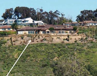
Natural vegetation has been thinned and/or replaced with fire resistant watered vegetation. This creates a buffer from direct flame impingement of the home. This buffer zone can vary in size depending on the location, vegetation threat, and construction type of the home.
