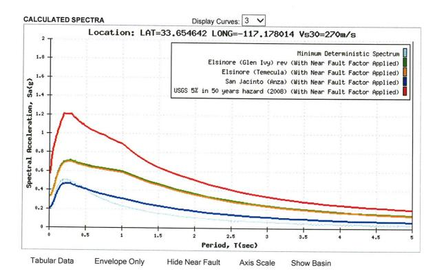
**Apply Near Fault Adjustment To:**NOTE: Caltrans SDC requires application of a Near Fault Adjustment factor for sites less than 25 km (Rrup) from the causative fault.
