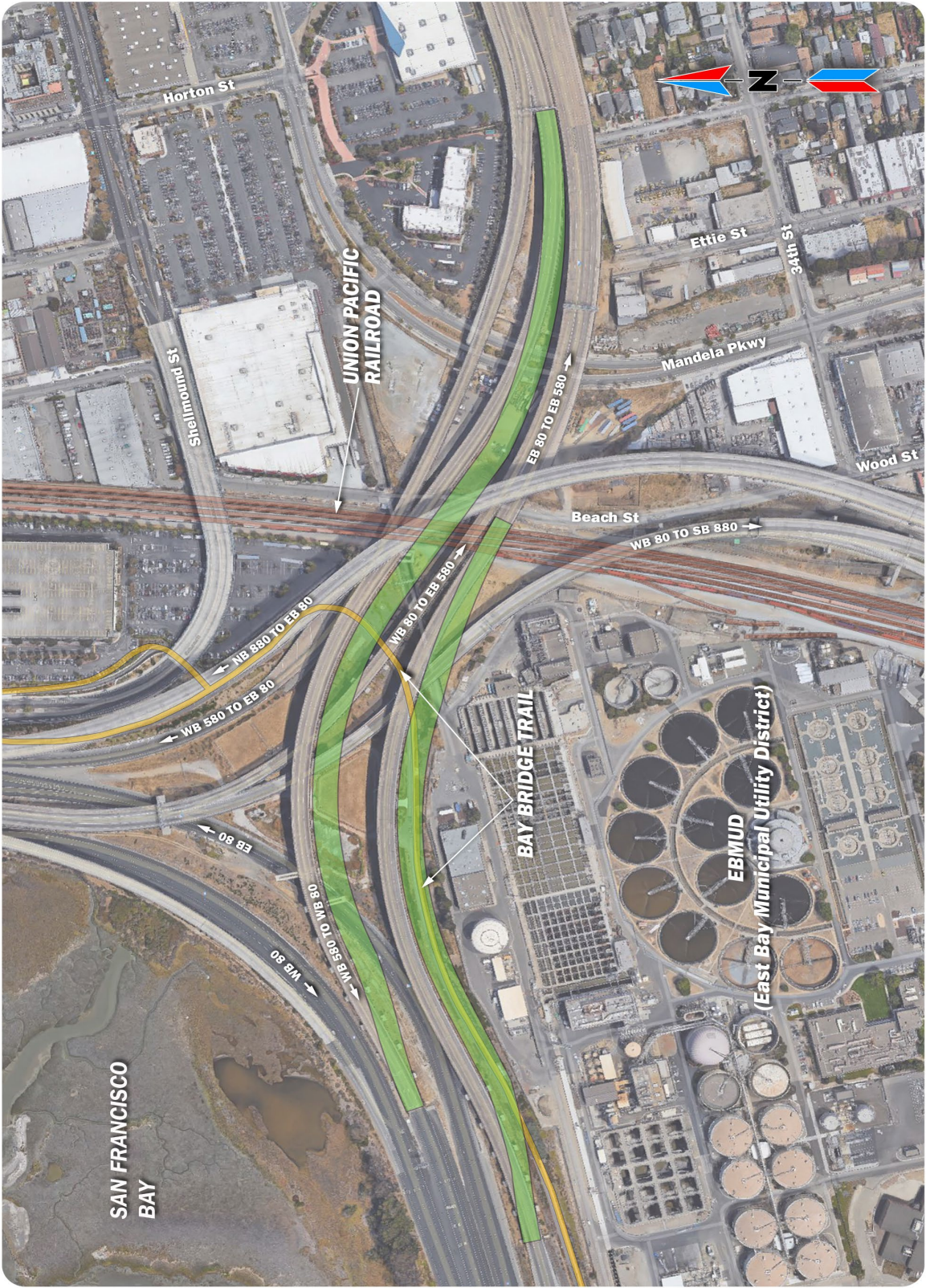
Figure 1-7 Alternative C: Partial Bridge Replacement
