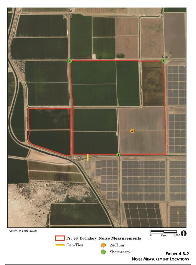
Measurement 2 was located at the northwest corner of the Project site, 50 feet south of the centerline of Kubler Road and 50 feet east of the centerline of Drew Road. During the measurement, seven passenger vehicles traveled along Drew Road. No traffic was observed on Kubler Road. The primary source of noise at this location was vehicle traffic on Drew Road.
