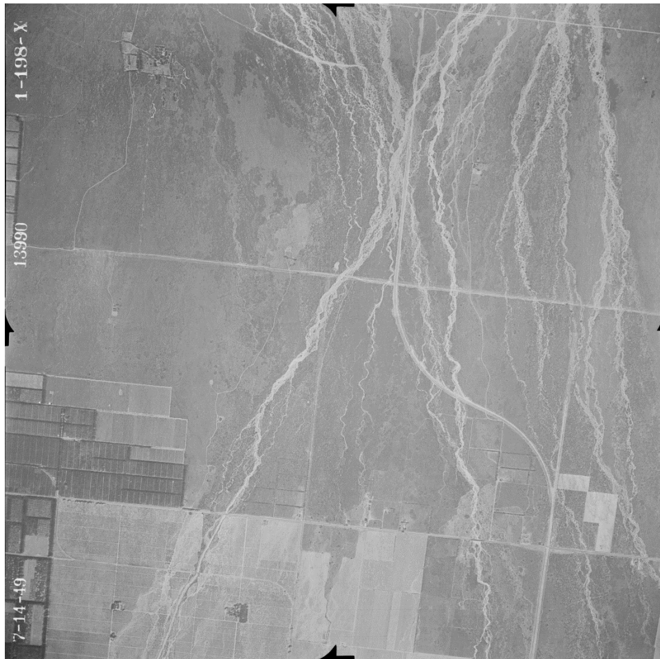
Figure 10 Fairchild Aerial Survey photograph of NPA showing “L-shaped” levee and earthen Day Creek Channel. Wilson Street bisects the middle of the photograph from left to right (FAS 1949)
