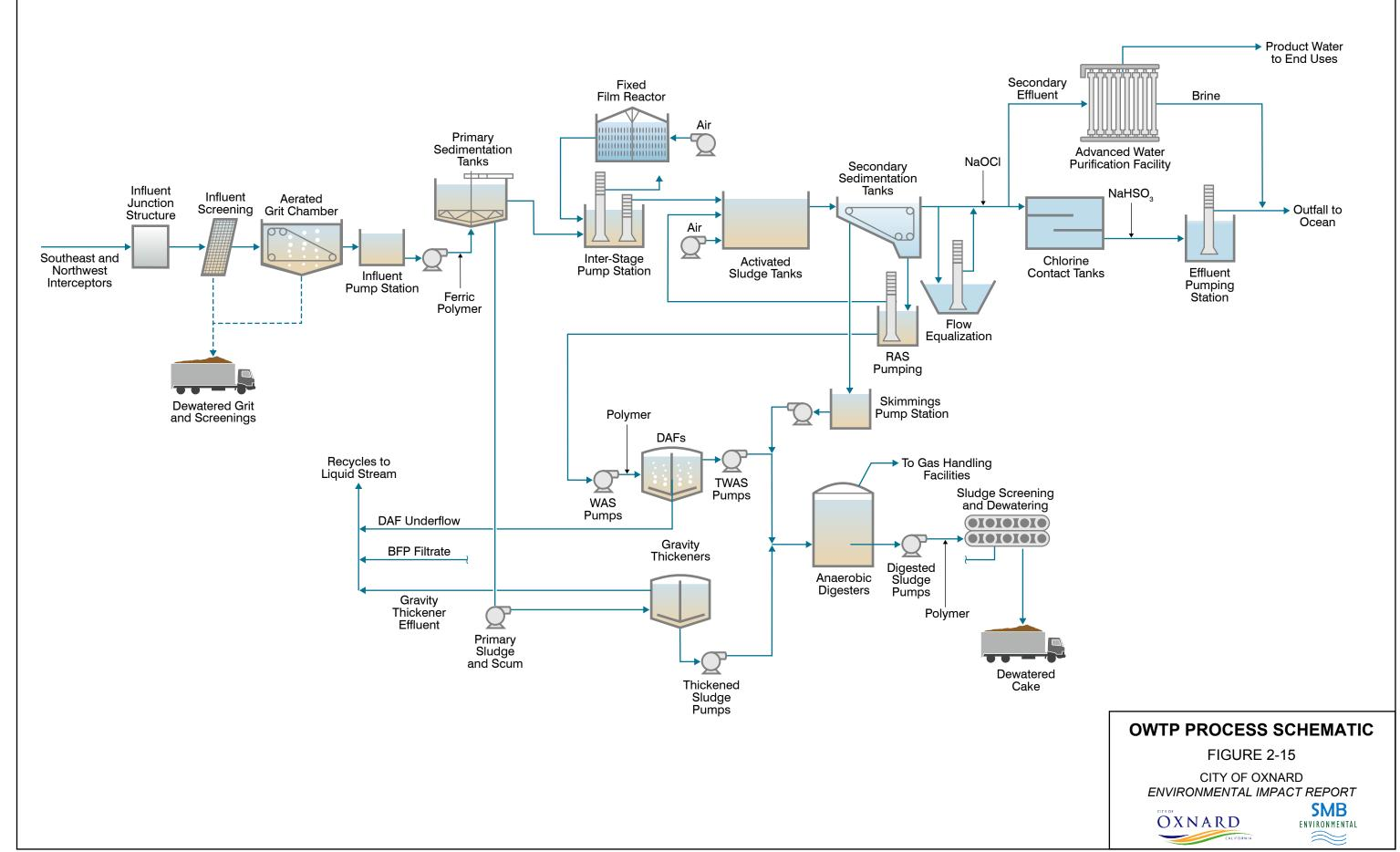
enhance sedimentation. A polymer storage and feed system is planned to further enhance primary treatment performance.
