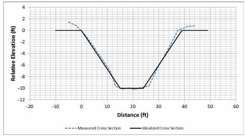
**Figure 4-1:** Idealized cross section, Camille Creek, based on a measured cross section at a carefully selected location.
