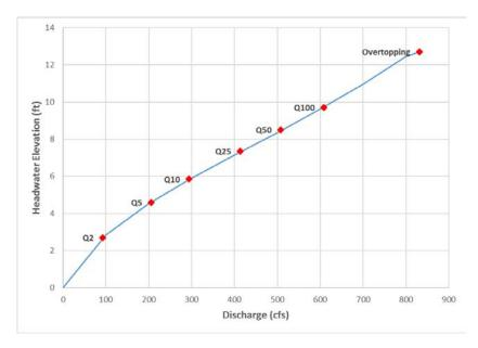
**Figure 6-4:** Stage-discharge rating for inlet of Sheehy Creek Hwy 29 culvert, obtained from HY-8 analysis. The red points show the water depth at the estimated recurrence interval peak flows.
