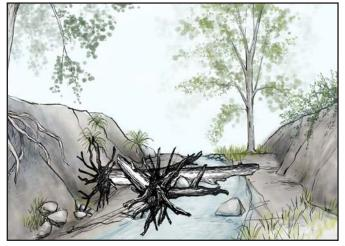
Photo 3. Downed tree, cut into smaller sections and repositioned in the channel to create instream complexity.
