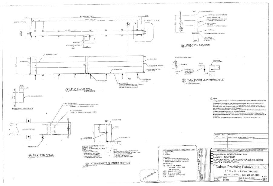
**Plate 1.7 - Stop Log Fabrication Drawing**
