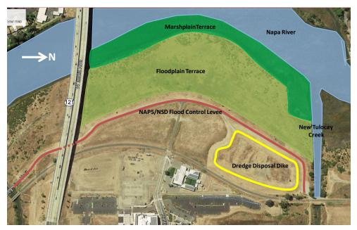
Figure 5-5: Site 2E - NSD Construction Features
