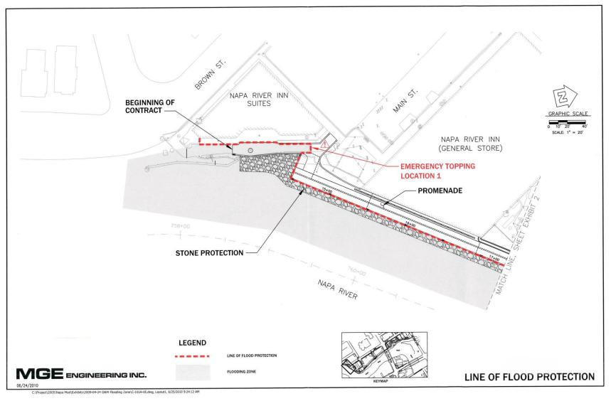
Plate 1.2 - Line of Flood Protection, Napa River Stations 758+00 to 760
