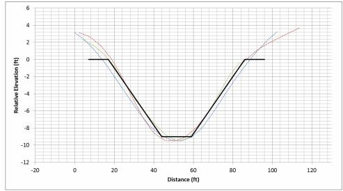
Figure 3. Idealized cross section, Tulucay Creek Reach 1, based on measured cross sections.
