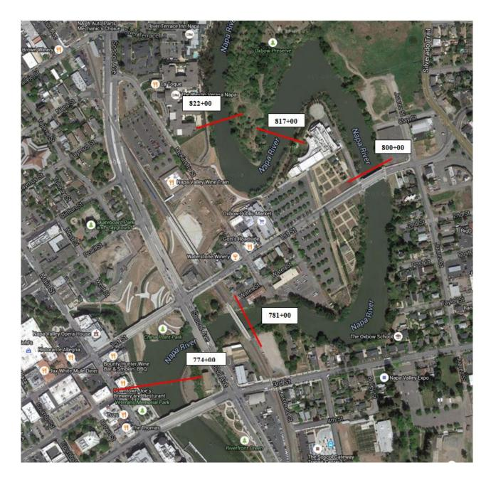
Figure 11-5: Permanent Survey Monitoring Cross Sections
