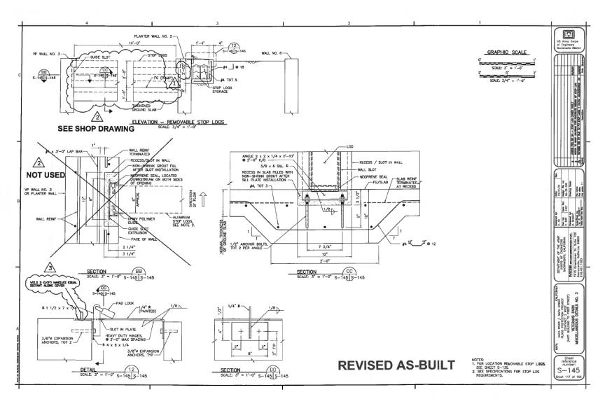
Plate 1.6 – Stop Log As-built drawing
