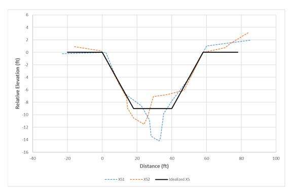
**Figure 5-3:** Idealized trapezoidal channel cross section for the maintained reach of Fagan Creek, overlaid on cross sections XS1 and XS2, shown looking downstream.
