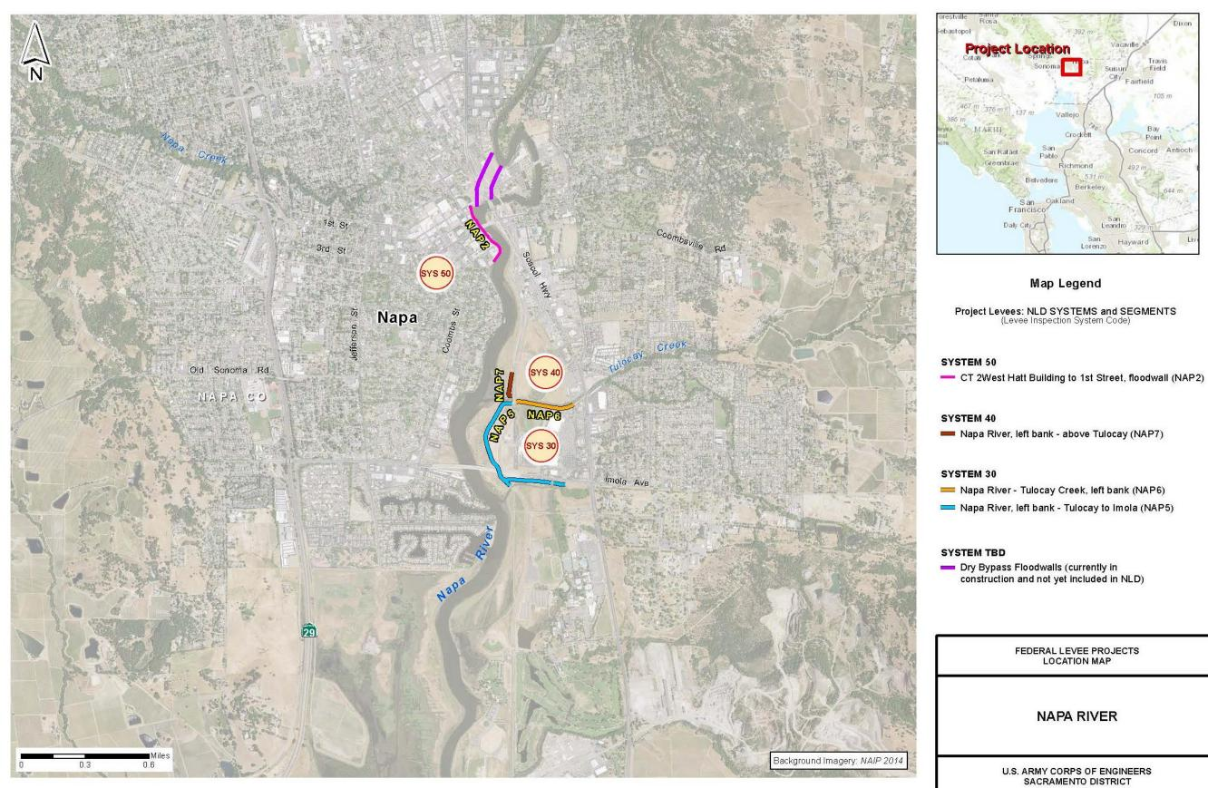
Figure 4-1: Napa Levee Safety System and Levee Inspection Program Map
