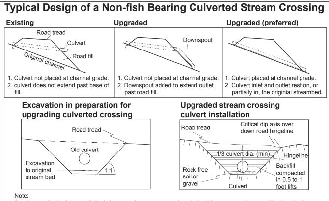
Road upgrading tasks typically include upgrading stream crossings by installing larger culverts and inlet protection (trash barriers) to prevent plugging. Culvert sizing for the 100-year peak storm flow should be determined by both field observation and calulations using a procedure such as the Rational Formula.
