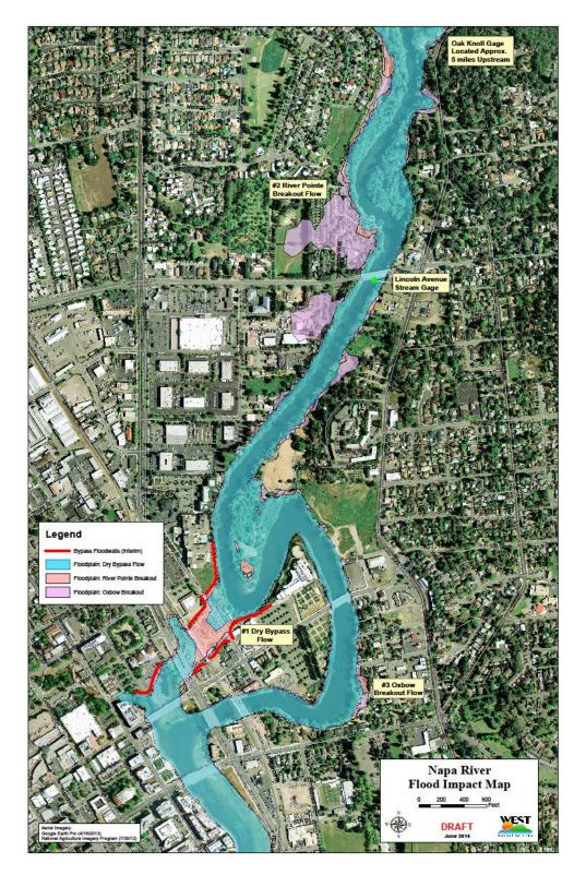
Figure 6-5: Anticipated Breakout Points when the Flood Events Exceed the Interim Condition for Napa River
