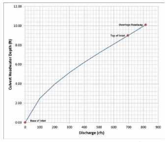
**Figure 4-3:** Headwater depth – discharge rating for South Terrace Drive culvert, obtained from HY-8 analysis.
