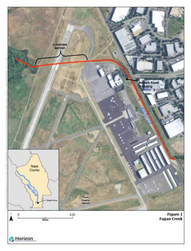
Map A. The upper 3,400 feet of the reach is open channel, which transitions to a 1,350-foot culverted section that flows underneath the airport runway, followed by 600 feet of open channel that discharges to Fagan Slough.
