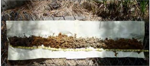
**Photo D-1B** – Soil profile at TSI-1 (SEZ). Soil is extensively mottled in upper part and becomes grayer at 19- to 35-inch depth.
