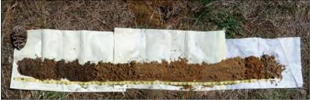
**Photo D-5B** – Soil profile at TSI-5 (SEZ). Soil profile indicates presence of old fill atop native soil (beginning at approximately 19 inches).
