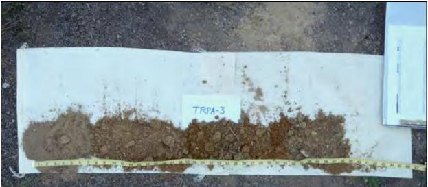
**Photo D-3B** – Soil profile at TSI-3 (SEZ). Soil profile indicates the upper 20 inches is fill material. The underlying soil appears to be truncated profile (topsoil removed before filled).
