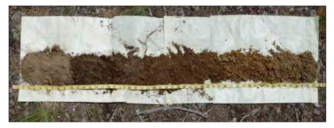
**Photo D-7B** – Soil profile at TSI-7 (Upland). While sample location was historically cleared (minor disturbance), profile indicates lack of extended wetness in upper 35 inches.
