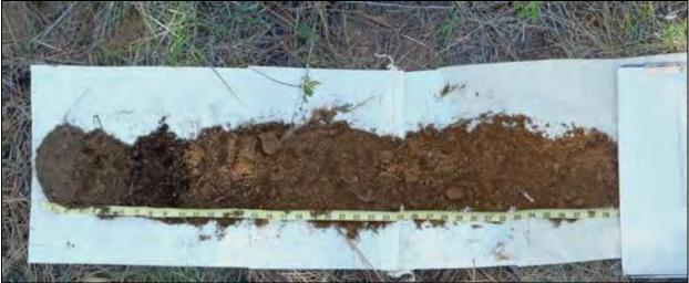
Photo D-10B – Soil profile at TSI-10 (Upland). Soil profile indicates lack of extended wetness within 39 inches of surface (rock refusal at 39 in.).
