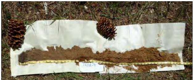
**Photo D-4B** – Soil profile at TSI-4 (Upland). Soil profile indicates no extended wetness in upper 49 inches.
