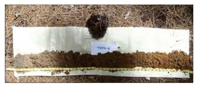
Photo D-6B – Soil profile at TSI-6 (Upland). Soil profile indicates lack of significant disturbance and lack of extended wetness in the upper 25 inches.
