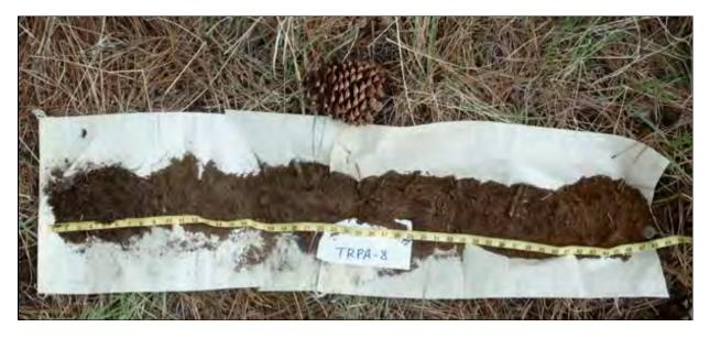
**Photo D-8B** – Soil profile at TSI-8 (Upland). While sample location has trees planted, profile appears undisturbed and lacks indication of extended wetness in upper 53 inches.
