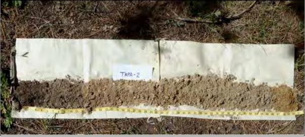
**Photo D-2B** – Soil profile at TSI-2 (SEZ). Soil profile indicates soil location was historically wetter, but plant community indicates drier current conditions.
