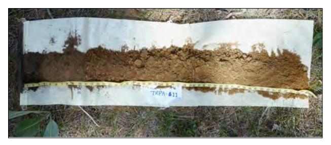
Photo D-11B – Soil profile at TSI-10 (Upland). Soil profile indicates lack of extended wetness within 40 inches of surface (2 to 20% iron RMFs from 40 to 53 in. depth)
