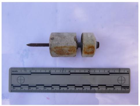
Photo 101-0146 TV-TF-ISO-01 ceramic insulator on ferrous wire nail. Detail. UTMs: 759680mE/4310714mN. Taken 08/24/16, T. Milliron.
