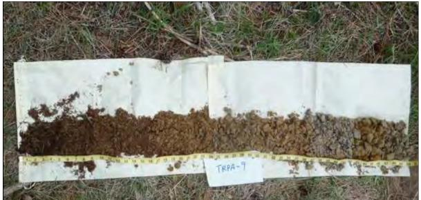
**Photo D-9B** – Soil profile at TSI-9 (SEZ). Soil profile indicates extended wetness rises to 24 inches, while plant community qualifies as SEZ. Hydrology monitoring recommended.
